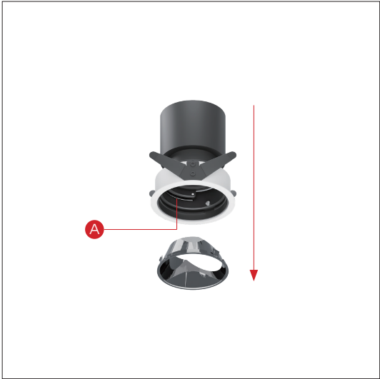
2. Take the pull ring out, as marking A, tilt angle horizontally with pull ring, which is more easily.
