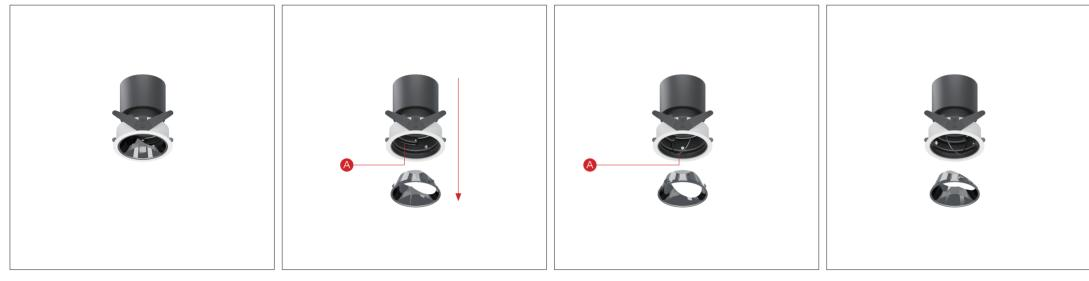
1. Remove the bottom reflector
