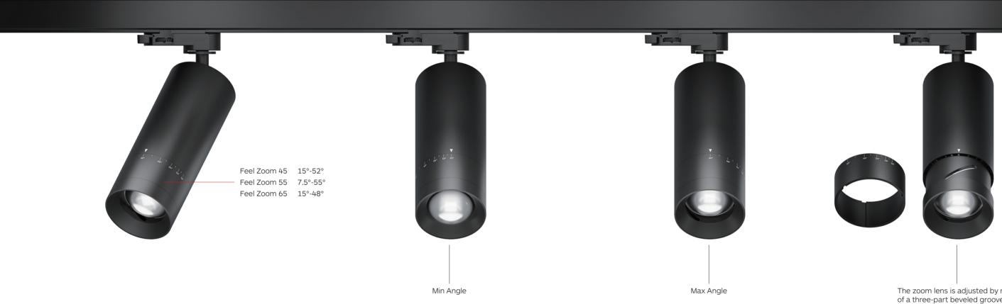
The zoom lens is adjusted by means of a three-part beveled groove (CNC machined) with a rotating ring. Min to maxi angle without changing the appearance of the luminaire.
